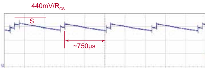
Fig.2. Short-circuit inductor current.
